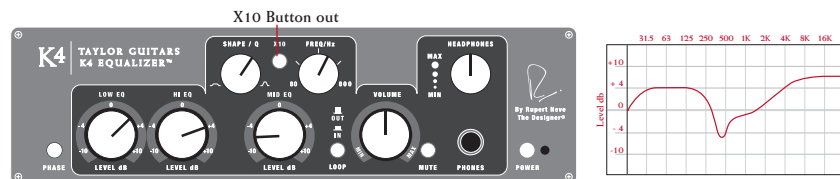
Mid cut setting and its effect on the signal
